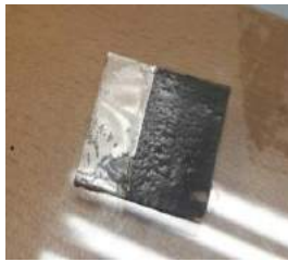
Figure 3.1 Conductive ink printed on the substrate
