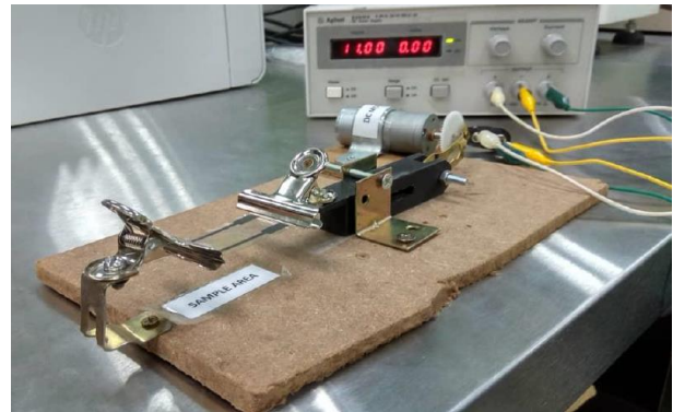
Figure 3.2 Fabricated cyclic bending test apparatus
