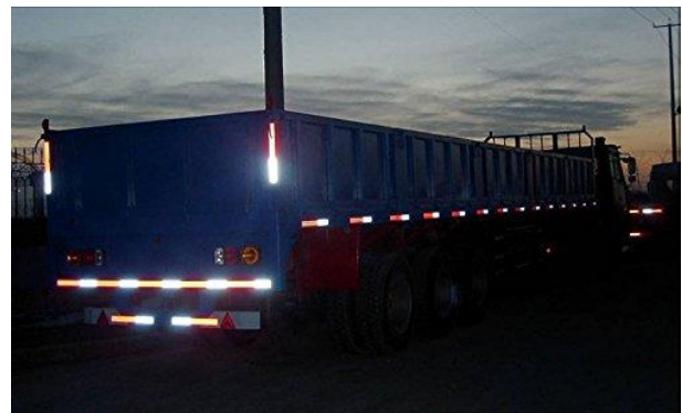
Figure 2.1 A trailer with extra lighting and stickers
