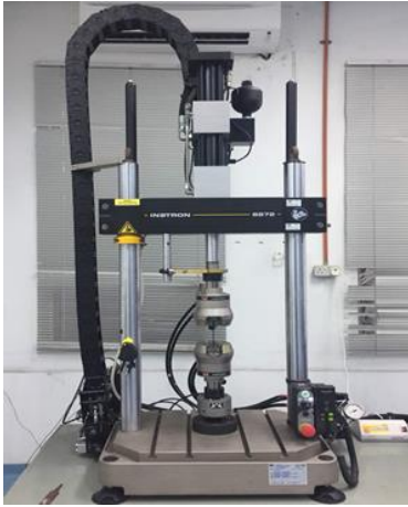
Figure 2.1 Universal Testing Machine, Instron 8872
