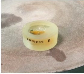
Figure 2.2 Sample that has been cold-mounted
