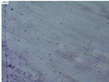
Figure 3.2 Morphological image of 10 % of filler loading on silver nanoparticles-filled epoxy
