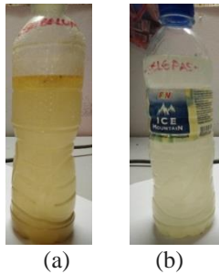
Figure 3.1 Wastewater quality (a) before, and (b) after installation of the oil trap system.
