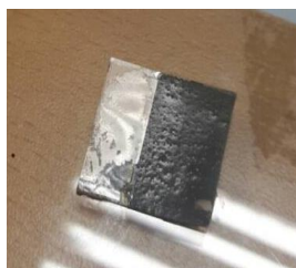
Figure 3.1 Conductive ink printed on the substrate
